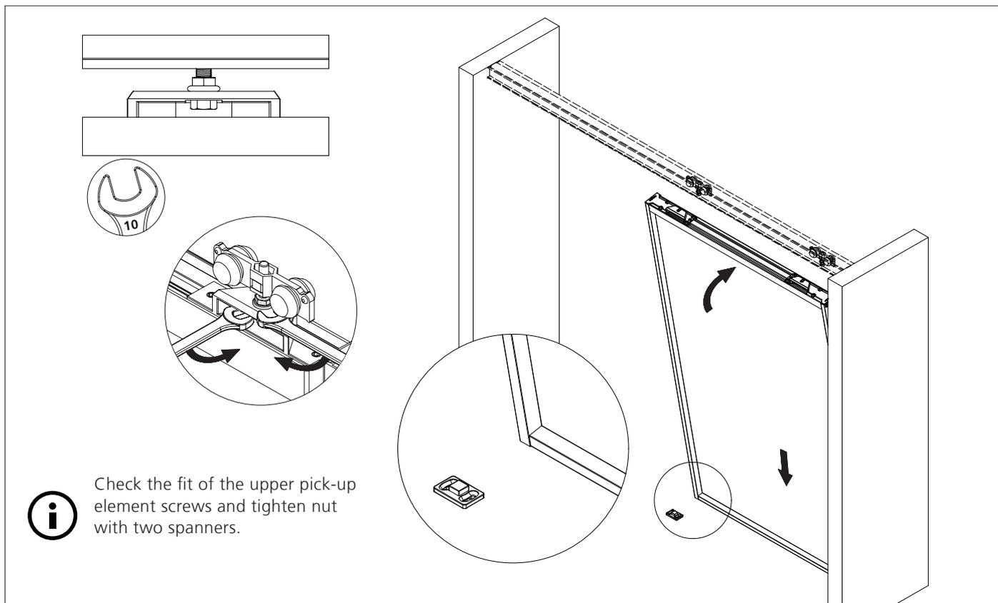
2\_ Install rear sliding door, then tighten the counter nuts at the pick-up elements.
