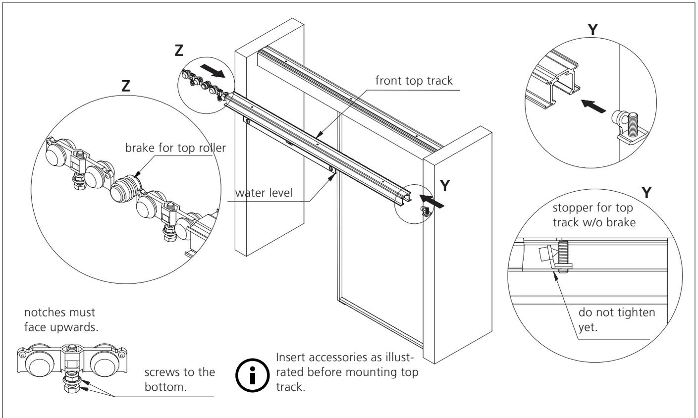
1\_ Drill holes in ceiling/top of corpus and mount front top track horizontally (fig. w/o ceiling/corpus).
