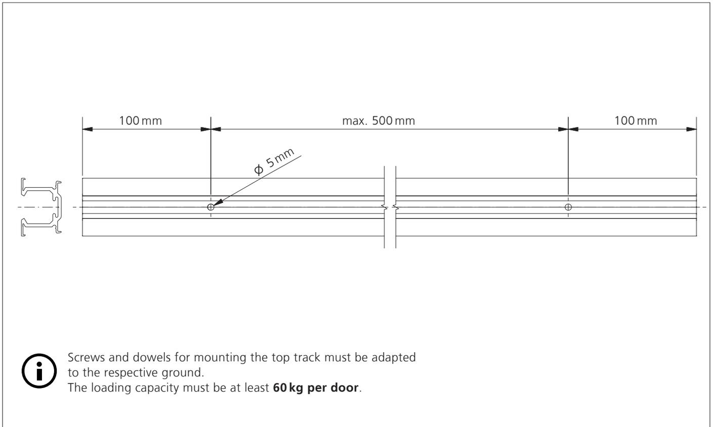
1\_ Cut cover for top track, middle insert profile and top track to size and drill holes in top track.
