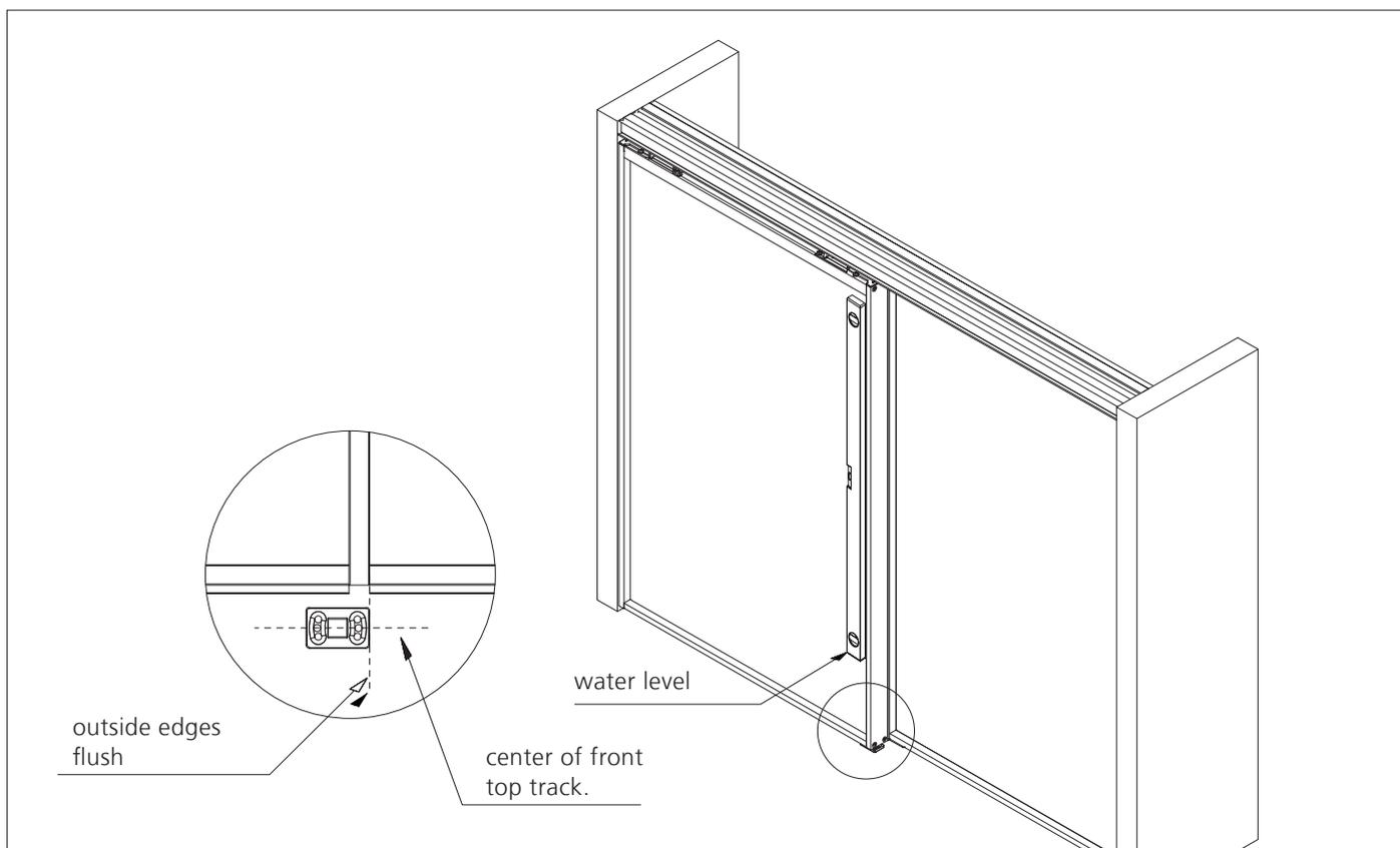
1\_ Mark position of ground plate (masking tape / pencil), unhinge front sliding door and mount ground plate.
