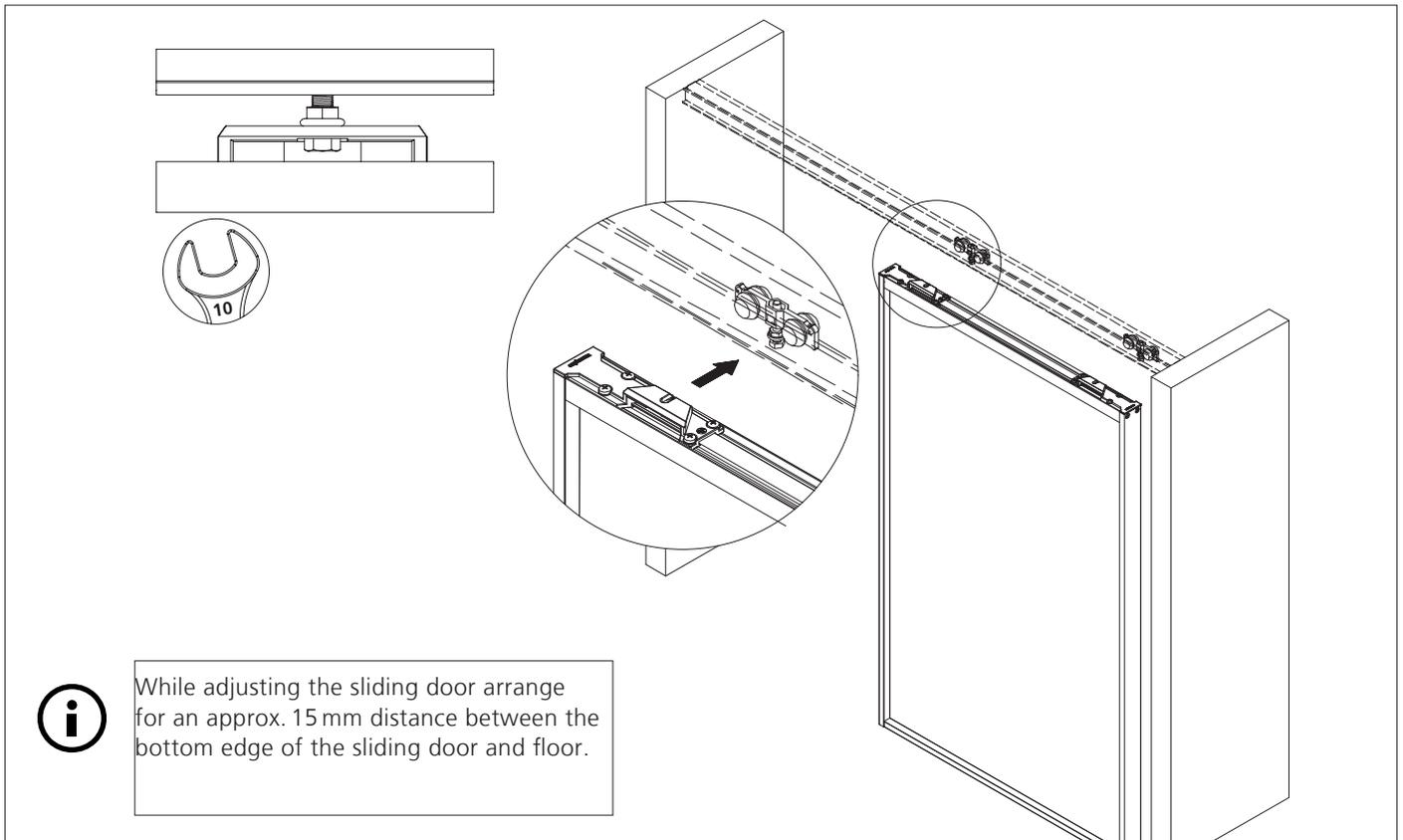
1\_ Install the **rear** sliding door and adjust perpendicularly with the set screws – **do not tighten yet.**
