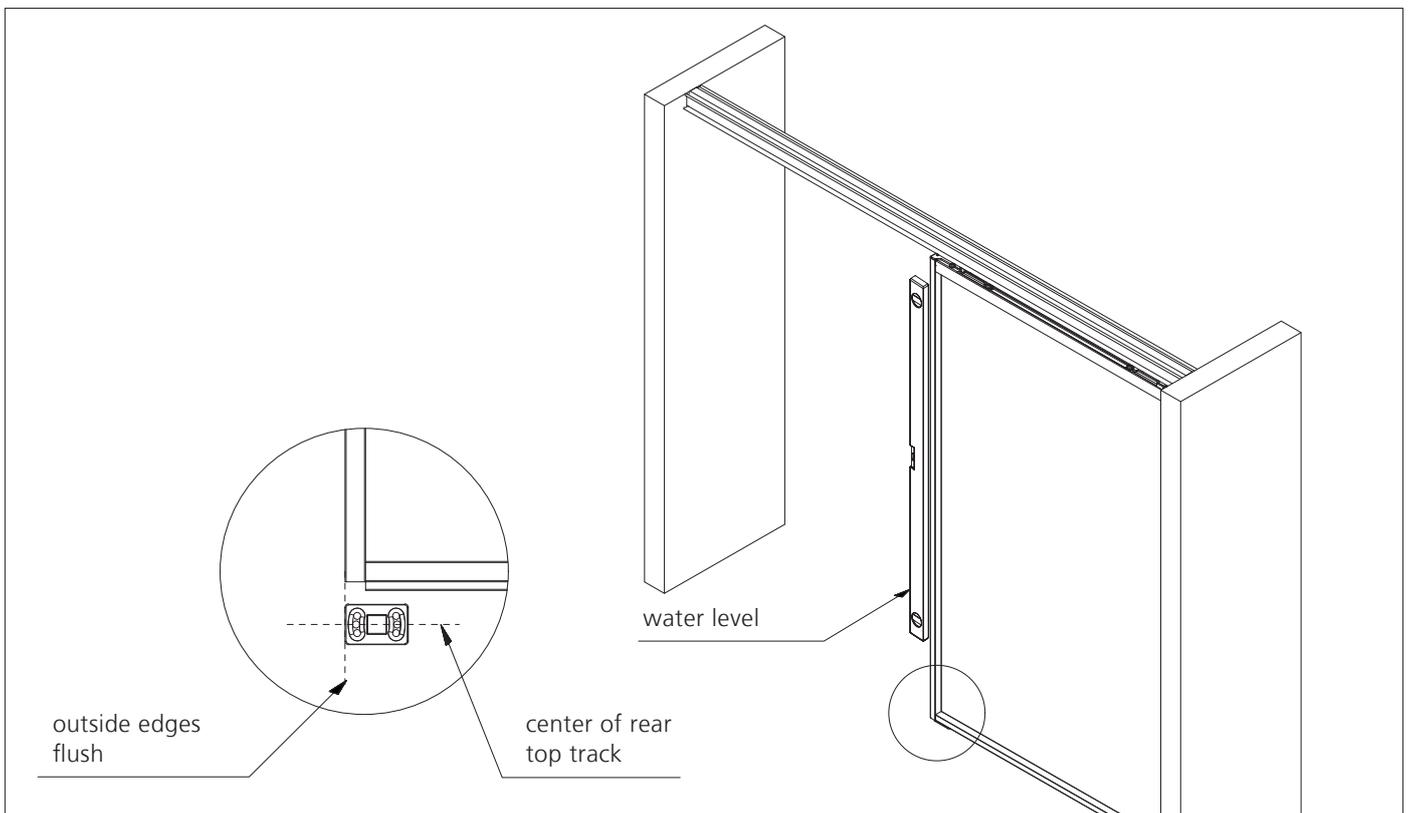
2\_ Mark position of ground plate (masking tape / pencil), unhinge rear sliding door and mount ground plate.
