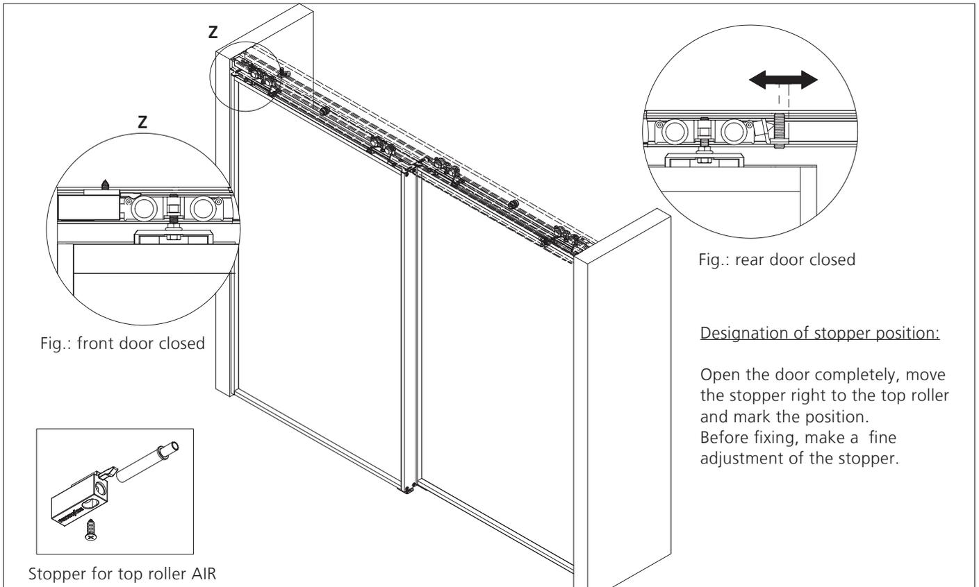
1\_ Mount stopper for top roller AIR in both top track inserts at closing positions.
