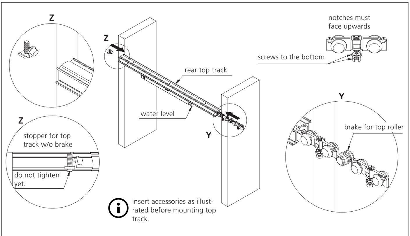
2\_ Drill holes in ceiling/top of corpus and mount the rear top track horizontally (fig. w/o ceiling/corpus).
