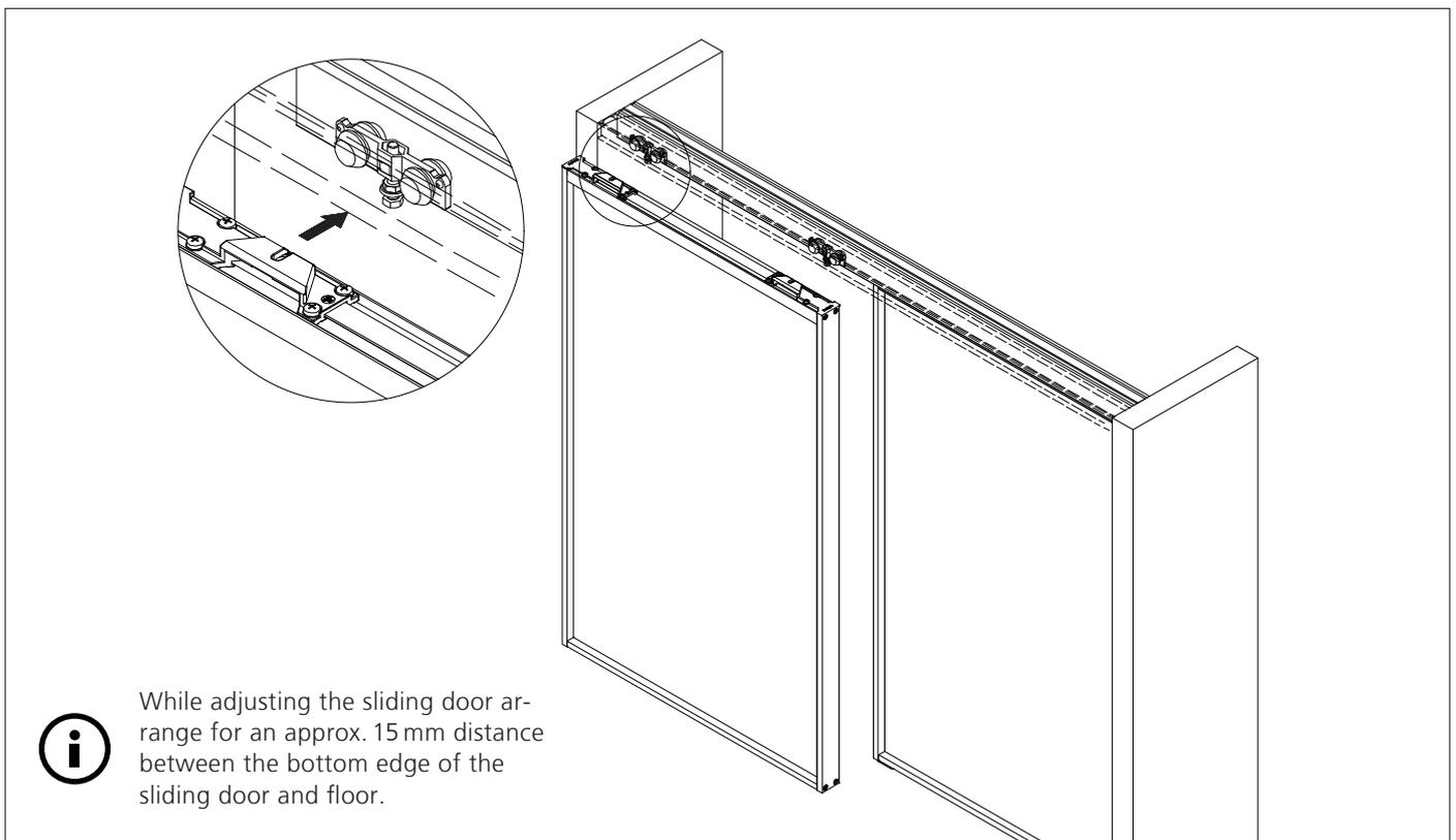
2\_ Install **front** sliding door and adjust perpendicularly with the set screws – **do not tighten yet.**
